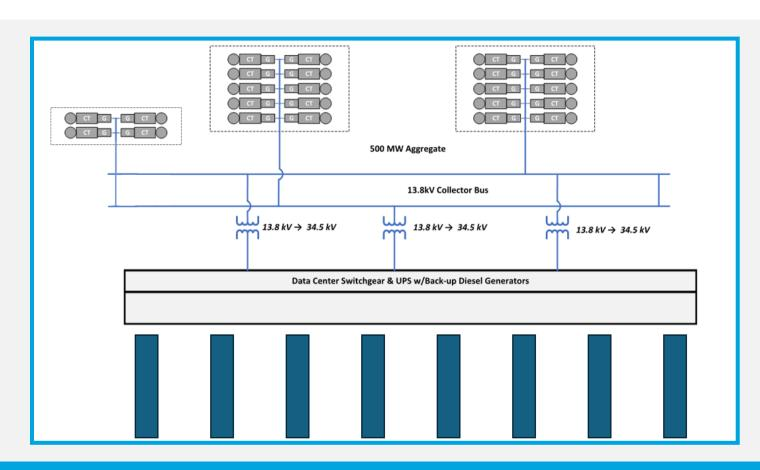
Reliability off the grid is directly proportional to the size of the largest unit; providing 20% redundant units increases reliability to 99.999% (the five 9s)
